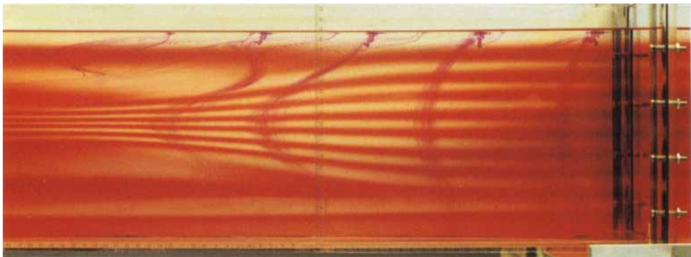
FIGURE 6. Internal self-similar flow (structure 2) with the withdrawal slit 11.5 cm above the bottom of the channel.
